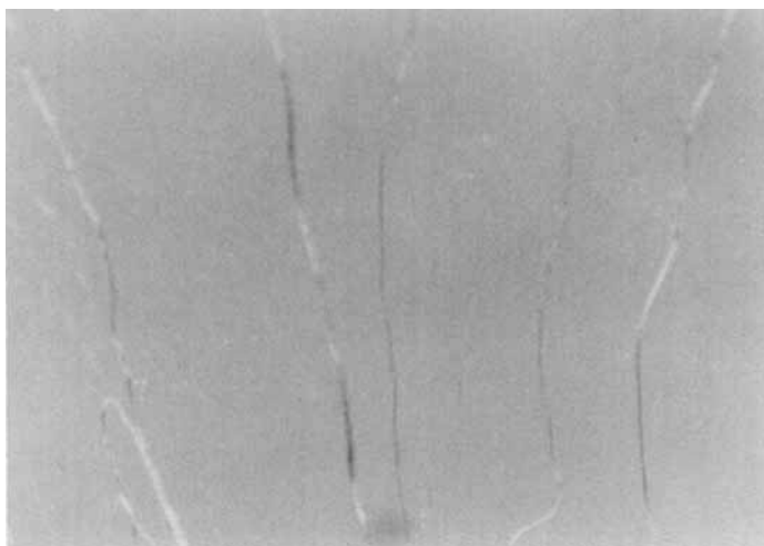
FIGURE 4 N^* , Cholesteric texture with oily streaks. Crossed polarizers, 136.5°C, X100. 5A. See Color Plate V.
